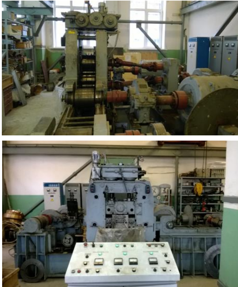
Fig. 1. General view of laboratory rolling mill - quarto and control console
