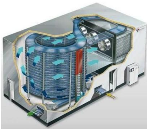
Figure 2 – Spiral quick freezer for freezing semi-finished dough products
