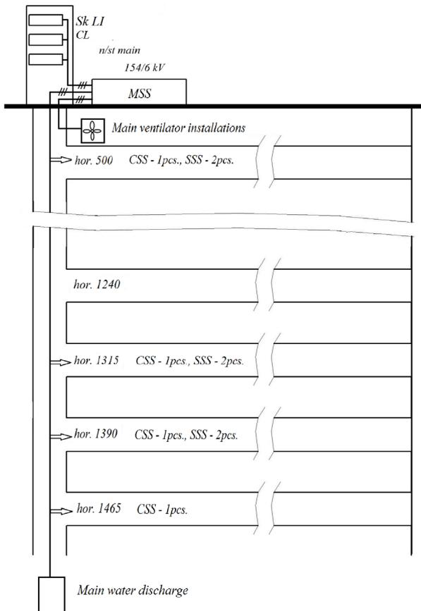
Fig. 3. Topology of electricity complex: electricity supply system – receivers of electric energy at an underground iron-ore company (a mine, an iron-ore mine): MSS – main step-down substation; CSS – central step-down substation; SSS – section step-down substation, SkLI – skip lifting installation, CL cage lift; hor. 500-1465 (underground horizons of respective depths (m) at the mine Ternivska (Ukraine)
